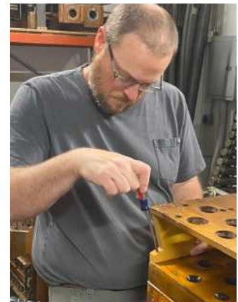
Tim Jones installing a new rack board top hat. This particular wood component had to be fabricated by Tim in his workshop.
