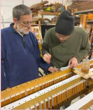
Scott Marsh and Tim Jones installing gaskets on the three rank chest.
