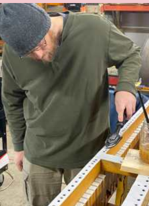
Tim Jones installing gaskets on the three rank chest.
