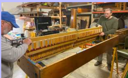
Brian Hunt and Tim Jones installing one of the interior secondary rank boards.
