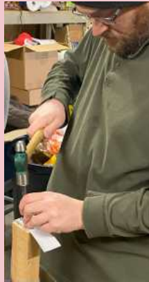
Tim Jones punching holes in the gasket material.
