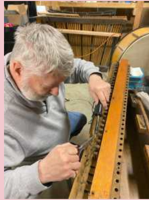
Brian Hunt unsoldering the old wiring from the bottom board.
