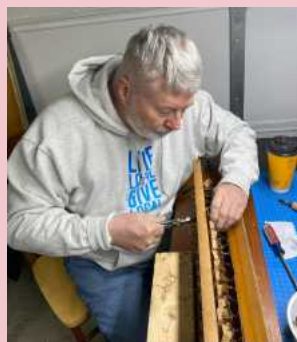
Brian Hunt removing old primary valves.
