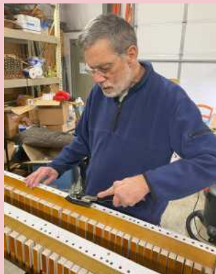
Scott Marsh installing gaskets on the three rank chest.
