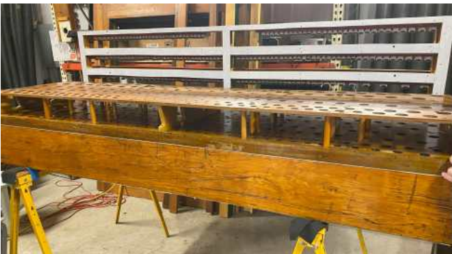
The three rank chest with the rack boards fitted in place prior to installing the pipes. The five rank chest is in the background with the new white leather gaskets.
