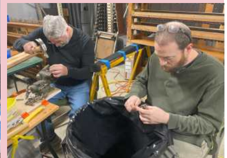
Brian Hunt removing the magnet caps and Tim Jones removing the old coil wiring.
