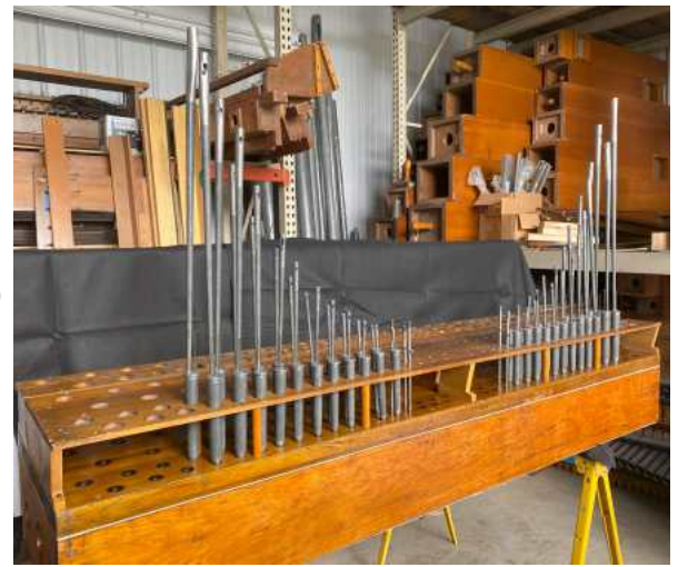
The three rank wind chest with the rack board assemblies fitted into place and a selection of the orchestral oboe pipes
