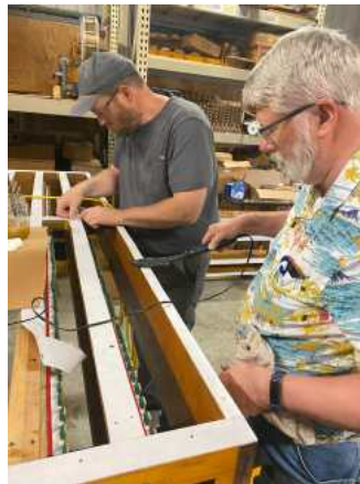
Tim Jones and Brian Hunt installing the new leather gaskets for the five rank chest
