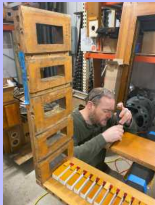
Tim Jones cleaning out the end board joint.
