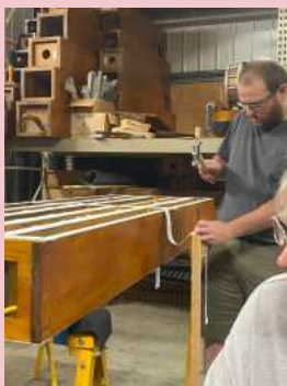
(Left and right): Tim Jones installing gaskets on the five rank chest
