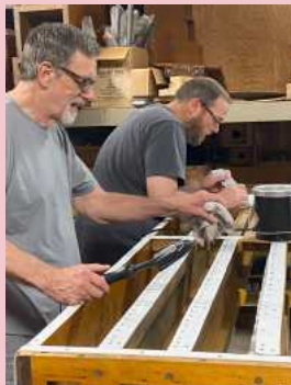
(left and right): Scott Marsh and Tim Jones installing gaskets on the five rank chest.
