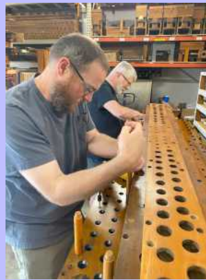
Tim Jones and Brian Hunt installing the toe boards.
