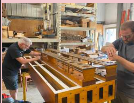
(left): Brian Hunt and Tim Jones installing rack boards on the five rank chest
