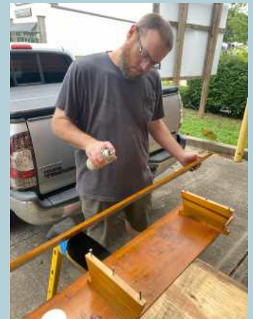
Tim Jones putting a coat of shellac on one of the bottom boards.
