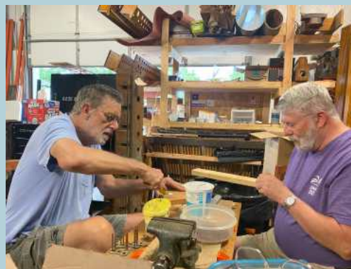
Scott Marsh and Brian Hunt removing old magnet coils from the magnet assemblies.
