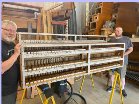
Brian Hunt and Tim Jones holding the three rank chest with all the gaskets installed
