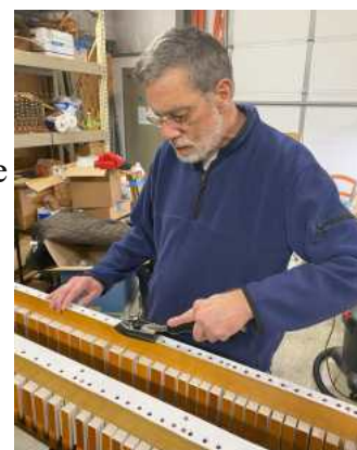
Heat setting the glue on new leather gaskets for the organ.
