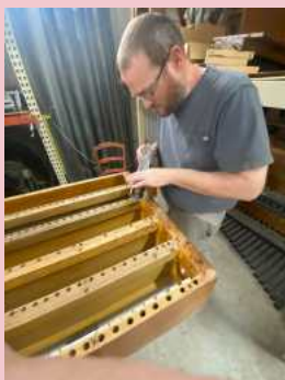
(Left and right): Tim Jones installing gaskets on the five rank chest
