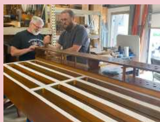
(above): Brian Hunt and Tim Jones installing the first rack board on the five rank chest.
