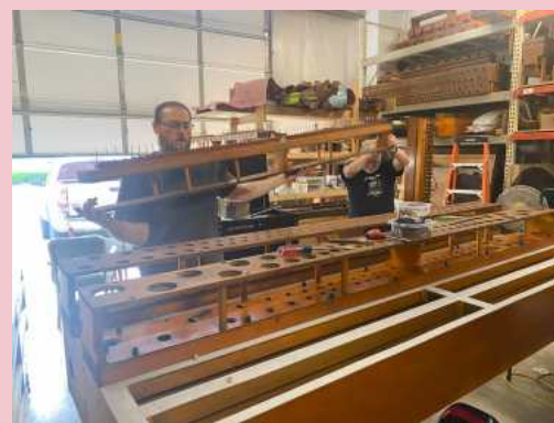
(right): Brian Hunt and Tim Jones installing rack boards on the five rank chest
