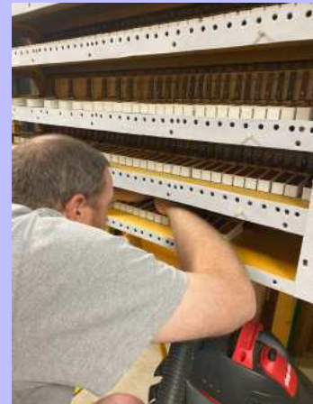
Two views of the new secondary valves and the refurbished pallet valves in the five rank chest
