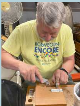
Brian Hunt removing old magnet coils from the magnet assemblies.
