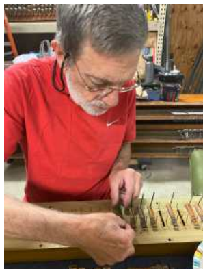
Installing new pallet valves on the organ
