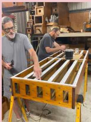
(left and right): Scott Marsh and Tim Jones installing gaskets on the five rank chest.
