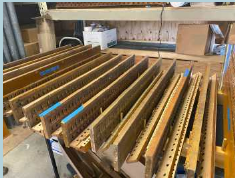
(above): to keep the individual wood components of the 16 bottom boards together, Tim designed and built a custom jig/ holder. It is working even better than expected.
