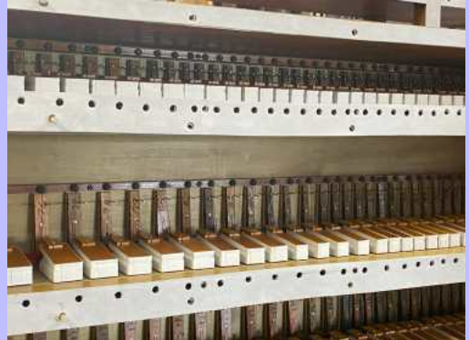
Two views of the new secondary valves and the refurbished pallet valves in the five rank chest
