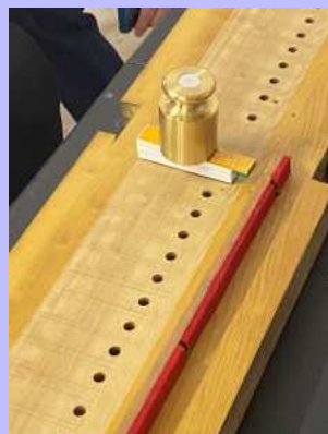
Using a weight to hold down the secondary valve until the glue sets.
