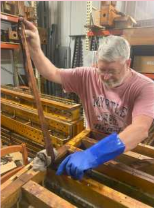
Brian Hunt removing the old gaskets from the five rank chest.
