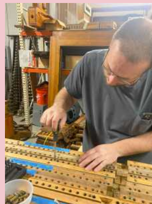
Tim Jones removing the threaded inserts.
