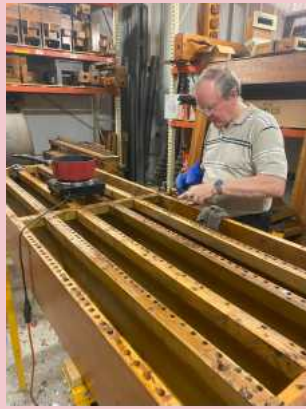
Dana Ross removing the old gaskets from the five rank chest.
