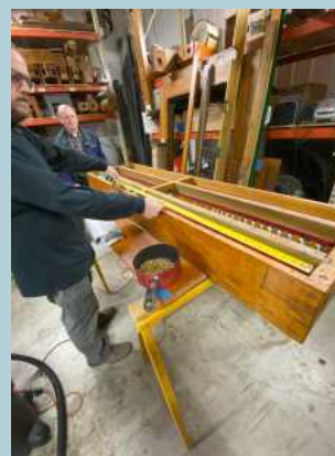
Tim Jones measuring the three rank chest for gasket leather.
