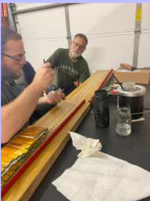
Tim Jones and Scott Marsh gluing secondary valves
