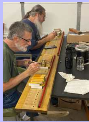
Scott Marsh and Garry gluing secondary valves onto the cabinet boards.
