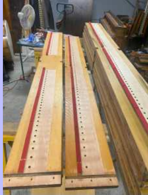
The refinished cabinet boards with the spring rails installed.
