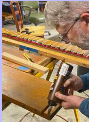
Brian Hunt gluing the end of the three rank chest
