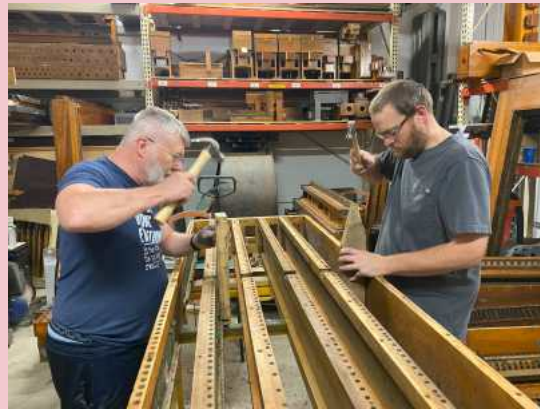
Brian Hunt and Tim Jones using their hammers to delicately dis-assemble the five rank chest.
