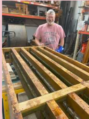
Brian Hunt and the five rank chest with all the old gaskets removed.
