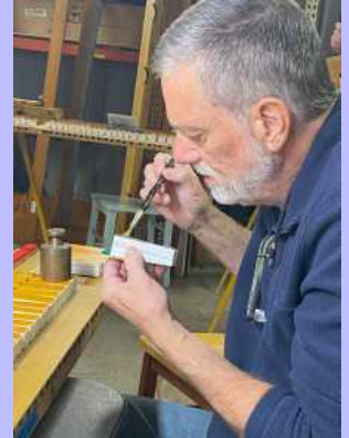
Scott Marsh gluing secondary valves on the cabinet board.
