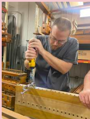
Tim Jones drilling out a dowel rod which didn't cooperate during dis-assembly.
