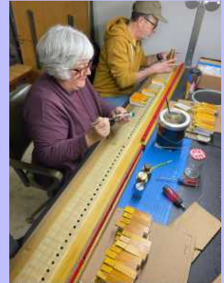
Lynn Vera and Pedro Vera gluing secondary valves onto the cabinet boards.
