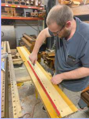
Tim Jones installing the spring rails on the cabinet boards.
