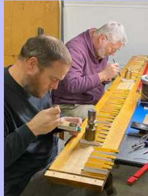
Tim Jones and Brian Hunt gluing secondary valves on the cabinet board.
