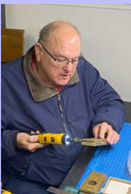
Jim Fitzpatrick using the jig to set the depth of the initial plastic nut on the wire.
