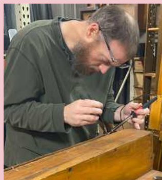
(left) Tim Jones unsoldering the long wire that runs the length of the chest
